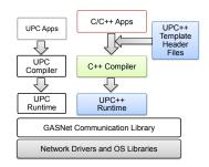
Fig. 2. UPC++ vs. UPC implementation stack
