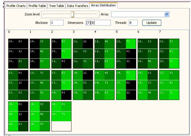
Figure 6. PPW Array Distribution visualization showing the physical layout of a 7x8 array with blocking factor of 3 on a system with 8 nodes
