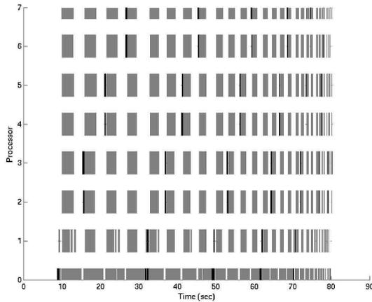
**Figure 4. Timeline for an LU run with no lookahead (SGI Altix Itanium 2 1.4GHz, n=12,800, process grid = 2x4, block size = 400). Grey blocks represent matrix multiplication and black blocks denote panel factorization.**
