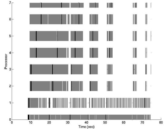
**Figure 5. Timeline for the same problem as Figure 4 with dynamic lookahead (a buffer size of 512MB). As a very small problem was used for illustrative purposes, the processors were not very busy towards the end of the computation.**
